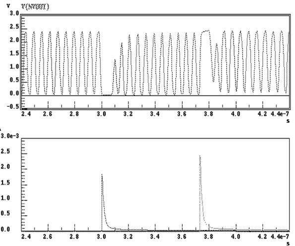
Figure 7. Example of VCO simulation with 2 impacts in the transistors of the second ring oscillator inverter. The first corresponds to the nmos impact and the second one to the pmos.
