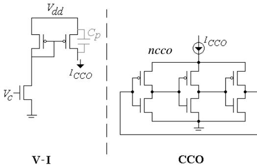
Figure 4. VCO schematic with output buffer
