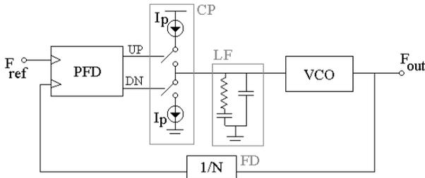
Figure 1. Charge-pump PLL
