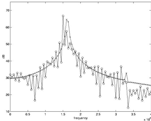
Figure 8. Frequency Spectrum for simulation of VCO under normal conditions (-x-) and under irradiation (-o-).
