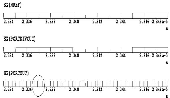
Figure 11. Digital inputs for PFD and VCO output after digitalization. The marked zone corresponds to Single Event in the output signal.
