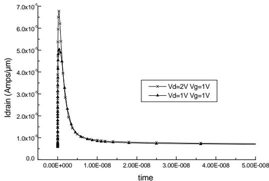
Figure 2. Transient currents for 2 different transistor biases in a FD SOI NMOSFET transistor with 2 $\mu\text{m}$  length. The particle is a  $^{132}\text{Xe}^{26+}$  and the impact is perpendicular to the channel.
