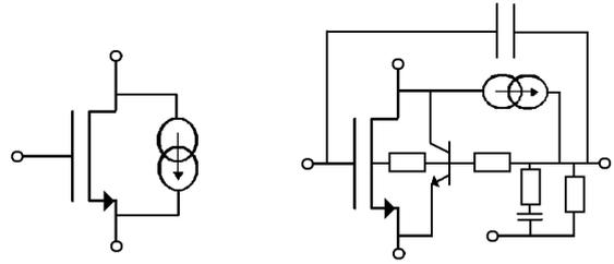
Figure 3. The left model represents the approach proposed in [11] . The right model is presented in [12].
