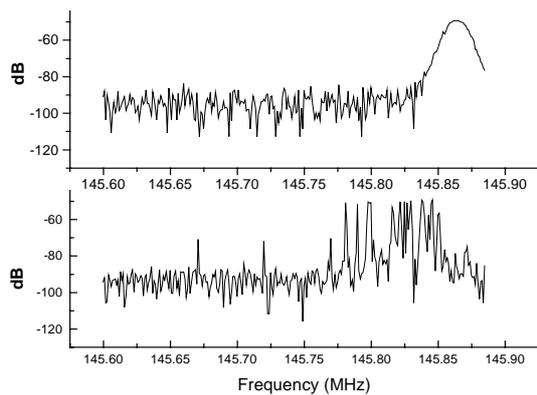
Figure 6. Frequency Spectrum of ring oscillator without radiation (top) and under large flux (bottom).
