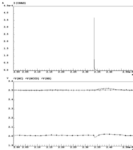
Figure 9. Irradiation current and voltages in the filter node (*nx*), VCO input (*Vc*) and CCO input (*ncco*)
