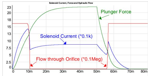
Figure 7: Solenoid Current, Force, and Hydraulic Flow
