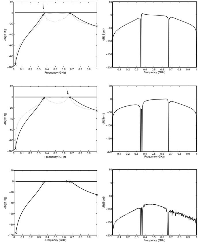
**Figure 4: Illustration of each step of the algorithm (when 4, 5 and 6 samples are selected). Magnitude Bandpass filter (full line) and best fitting model (dotted line) at left. The real fitting error at right. Accuracy fit : -82.4049 dB**
