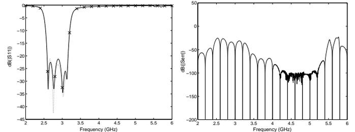
**Figure 1:** Magnitude Lowpass filter (full line) and fitting model (dotted line) with uniform sampling distribution at left. Complex error between fitting model and verification data at right. Accuracy fit : **-22.9730 dB**
