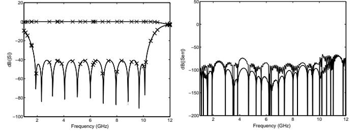
Figure 5: Magnitude data from different ports Quarter Wavelength filter (full lines) and fitting models (dotted lines) at left. Real error of all fitting models at right. Selected samples are marked with a cross. Accuracy fits : -65.9112 dB
