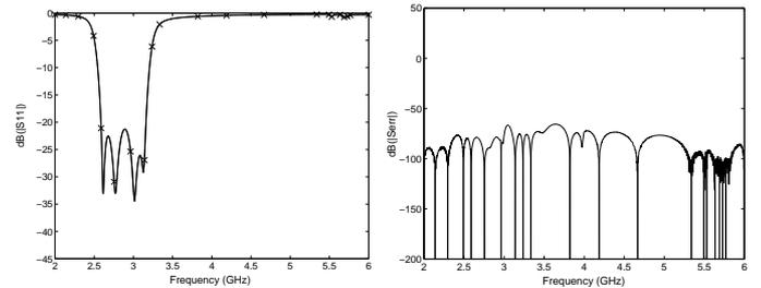
**Figure 2:** Magnitude Lowpass filter (full line) and fitting model (dotted line) with adaptive sampling distribution at left. Complex error between fitting model and verification data at right. Accuracy fit : **-65.6536 dB**
