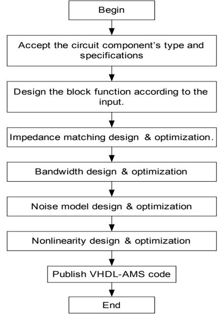
Figure 2: The design flow for behavioral modeling RF amplifiers and mixers
