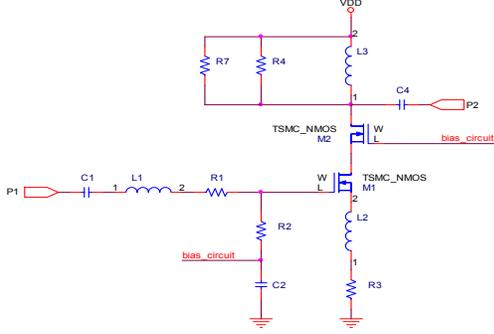
Figure 4: The schematic of a 1.9GHz LNA in TSMC25 technology
