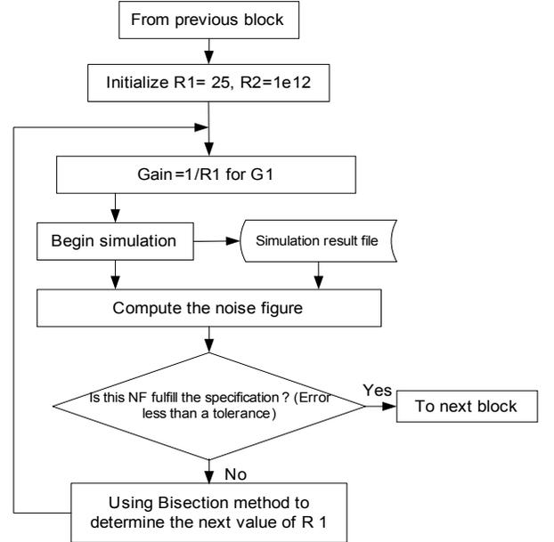
Figure 3: The design flow of noise modeling block
