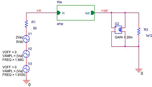
Figure 5: The test circuit of the LNA
