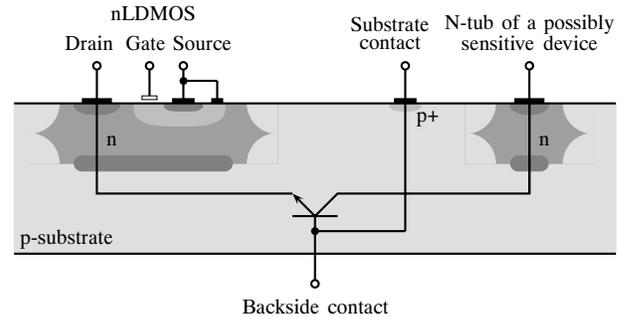
Fig. 1. Simplified cross section of a smart power IC showing the parasitic transistor.
