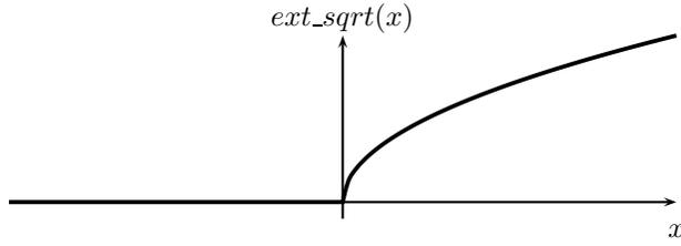
Fig. 3. Extended square root function
