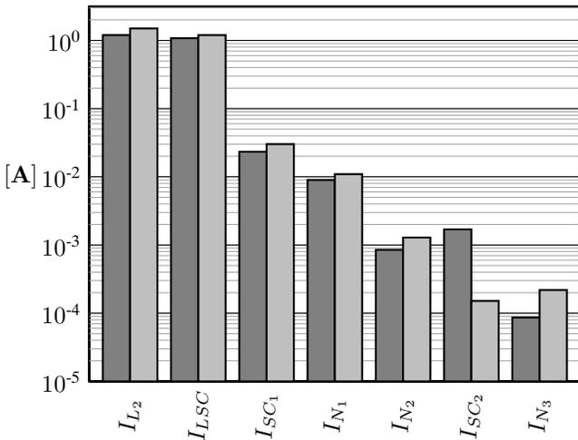
Fig. 10. Further simulation results of the structure in Fig. 6 for  $V_{L_2} = -1.5V$  showing selected currents from device simulation (gray bars) and circuit simulation (lightgray bars).
