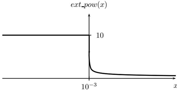
Fig. 5. Extended pow(x,-0.33) function
