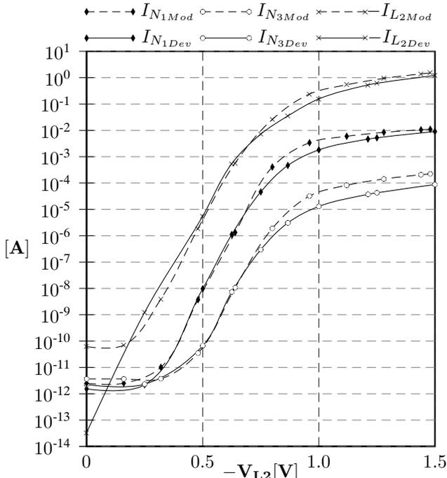
Fig. 9. Simulation results from device simulation (index  $Dev$ ) and circuit simulation employing the new model (index  $Mod$ ).
