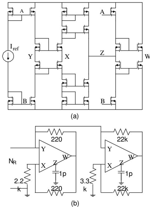
Figure 3: (a) Synthesis of a CFOA by cascading a CCII+ with a VF, and (b) its application to implement Chua's diode.
