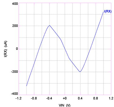
Figure 4: I-V characteristic of  $N_R$  implemented as shown by Fig. 3(b).
