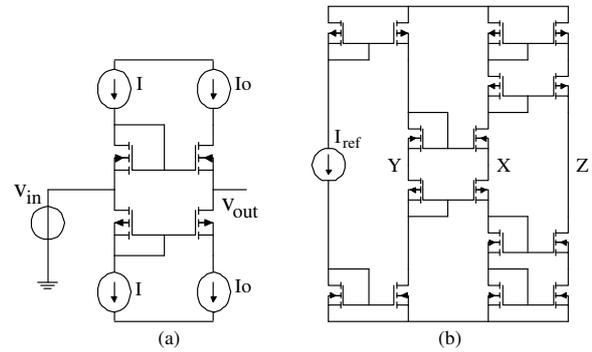
Figure 1: (a) VF biased with ideal current sources, and (b) synthesis of the biases to generate a CCII+
