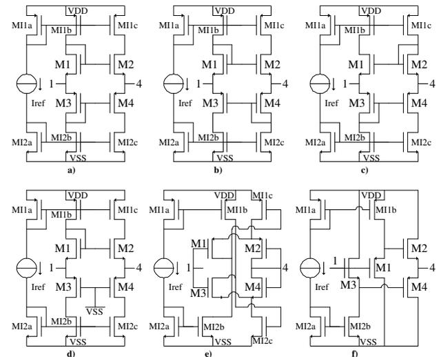
Figure 2: CMOS VFs synthesized from [7].
