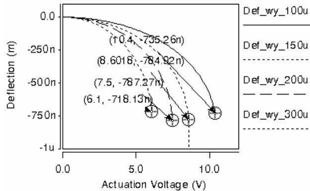
**Figure 6: The pull down voltage simulation in CoventorWare for 200 μm long and 100 μm wide beam at anchor.**
