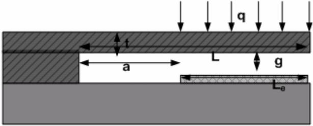
Figure 2: Side view of a non uniform cantilever
