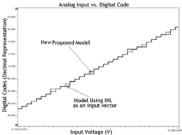
**Figure 6. A comparison between the transfer functions of a 16-**
