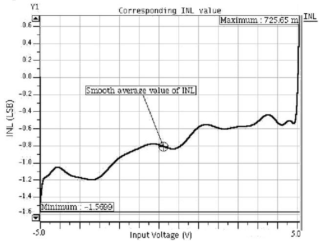
**Figure 7. The INL value calculated from the new model.**
