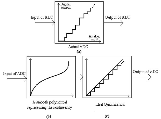
**Figure 3. The decomposition of the transfer function of the ADC. (a) The nonlinear actual transfer function of the ADC. (b) The smooth polynomial block. (c) The ideal quantization block.**
