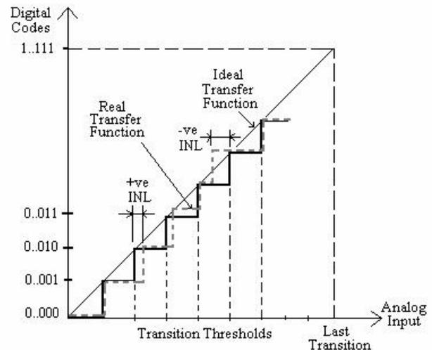
Figure 1. Transfer function of ADCs showing the INL
