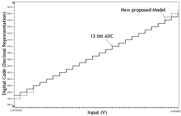
**Figure 5. A comparison between a 12-bit ADC Spice circuit and the output from the proposed behavioral model.**
