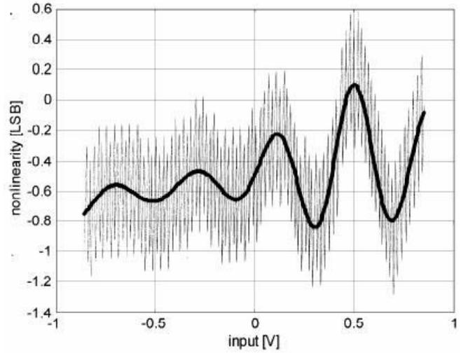
**Figure 2. A general figure for the INL of an ADC chip [5]**
