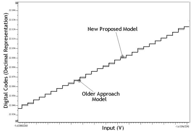
**Figure 8. A comparison between the two models stimulated by a sinusoidal input.**
