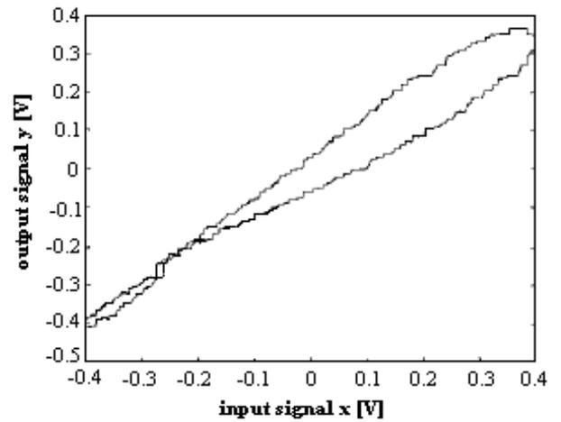
Figure. 4. Dynamic Response of an ADC using a sinusoidal input [6].
