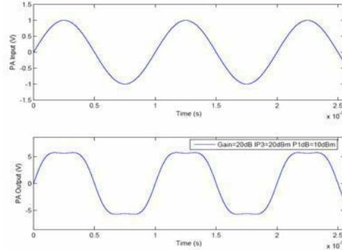
Fig.8. PA nonlinearity simulation
