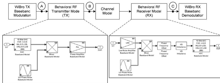
Fig.12. Mobile WiMax system implemented in Simulink with behavioral baseband equivalent model of RF transceiver.
