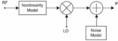
Fig.5. Mixer baseband equivalent model
