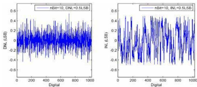
Fig.11. DNL and INL Characteristic for 10-bits converter
