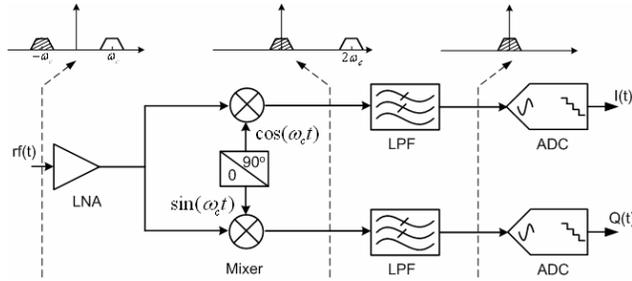
**Fig. 2. Direct-conversion receiver diagram and signal complex spectrum.**
