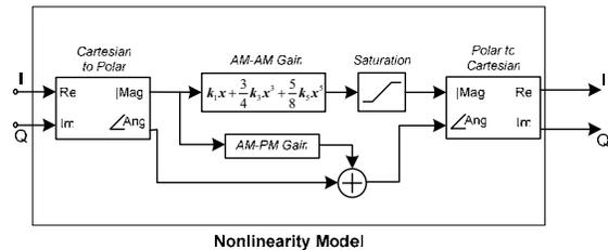
Fig.4. PA complex baseband equivalent model
