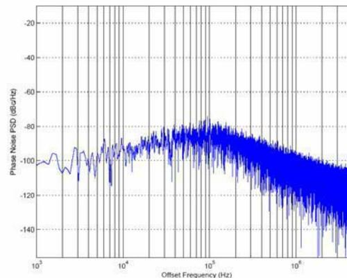
Fig.10. Simulated local oscillator phase noise with PLL
