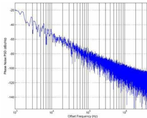
Fig.9. Simulated local oscillator phase noise without PLL
