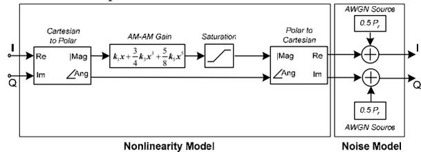
Fig.3. LNA complex baseband equivalent model
