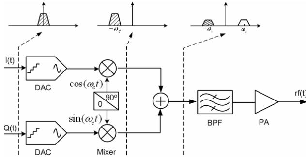
**Fig. 1. Direct-conversion transmitter diagram and signal complex spectrum.**
