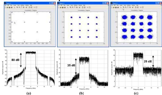
Fig.13. Wibro 16QAM Signal Constellation and Spectrum (a) Ideal signal source (b) Transmitted signal after PA (c) Received signal after ADC.
