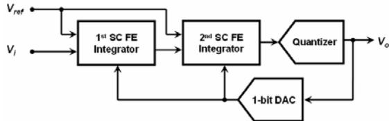
Figure 2. Second-Order SC  $\Delta\Sigma$  Modulator
