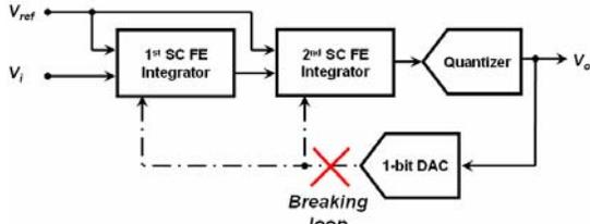
Figure 7. Extraction Mode of Second-Order SC  $\Delta\Sigma$  modulator
