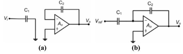
Figure 4. Operation Mode (a) Sampling (b) Integration
