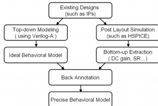
Figure 1. Bottom-Up Modeling Flow for Existing Designs
