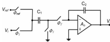
Figure 3. Single-ended Configuration of SC FE Integrator
