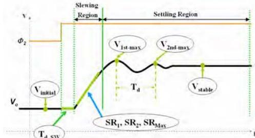
Figure 9. The Required Parameters of Settling Response
