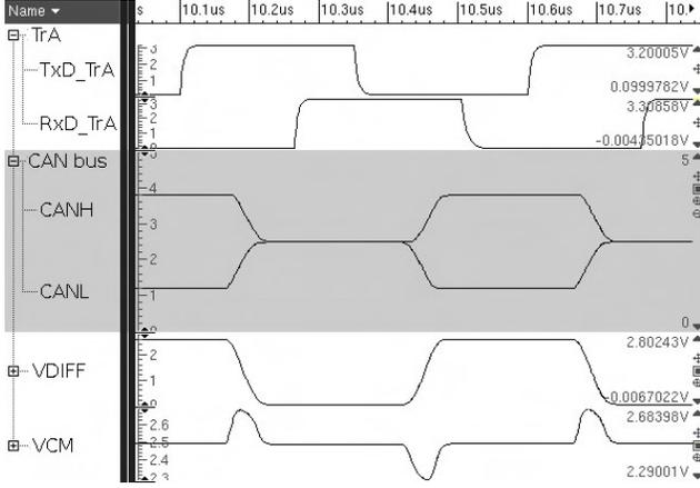
**Figure 4: CANH and CANL signal integrity analysis using the ACCURATE model architecture**
