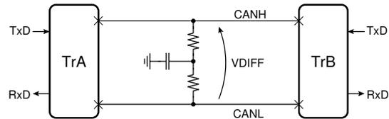
Figure 3: Network setup structure used for the transient analysis
