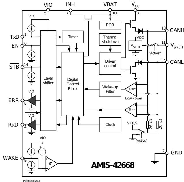
**Figure 1: AMIS-42668 CAN transceiver block diagram**
