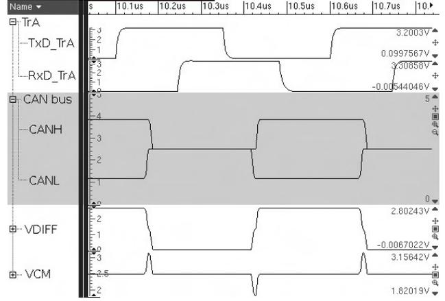
**Figure 5: CANH and CANL signal integrity analysis using the FAST model architecture**
