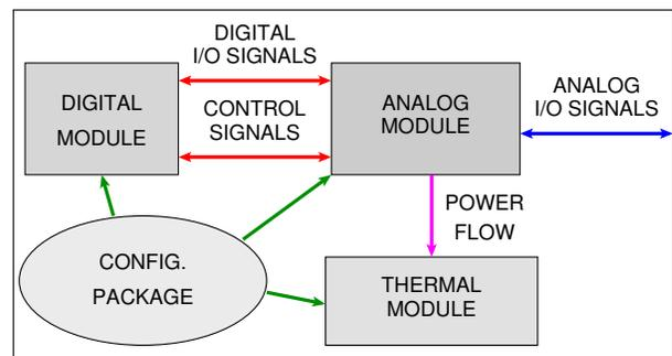
**Figure 2: CAN transceiver Mixed-Mode behavioral model block diagram**
