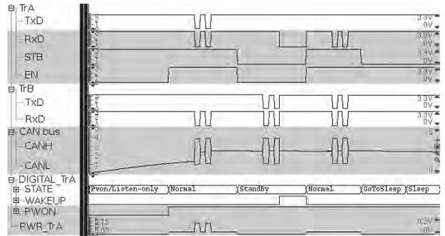
**Figure 6: Internal states hopping and remote wakeup analysis**
