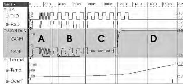
Figure 7: CAN bus short-circuit analysis
