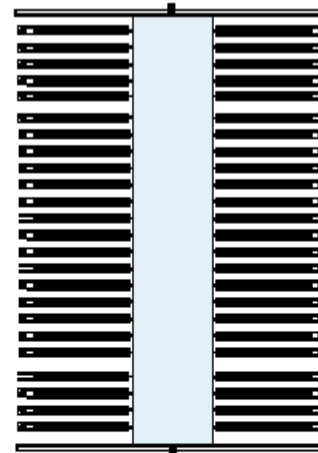
(b) Optimization design of experiment 1 (Static sensitivity optimized design) SNR=30.4dBdB Static Sensitivity=72fF/g
