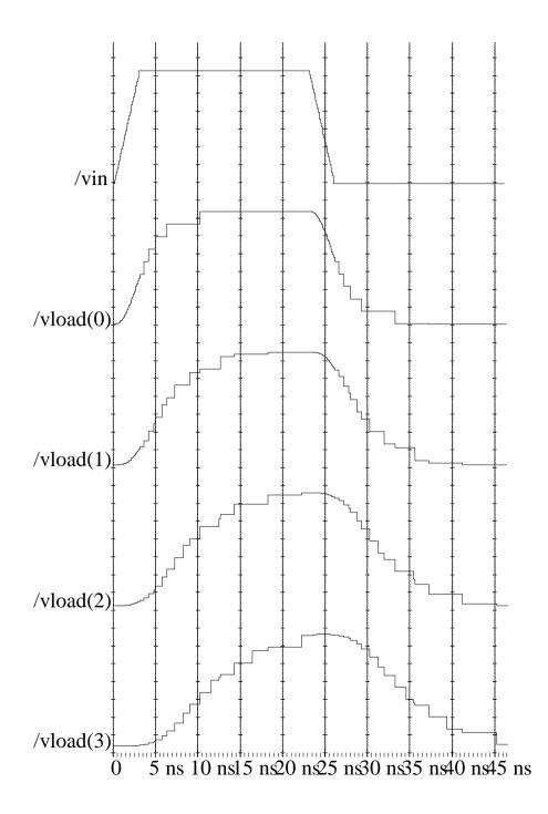
P Simulation results for a interconnection modeled using real poles
