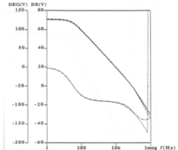
Figure 6. Frequency response curves (magnitude and phase) of the op-amp and its behavioral model.
