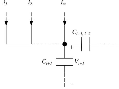
Figure 4. General node in an analog circuit.
