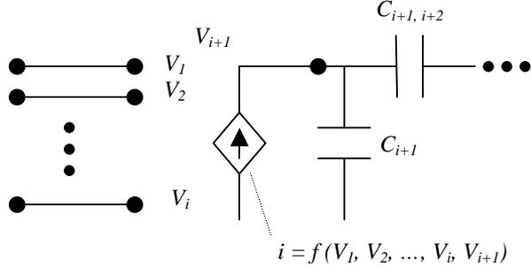
Figure 3. General representation of a physically modeled node.
