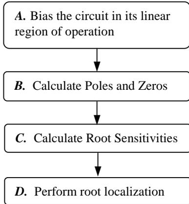
Figure 2. Analyses performed on linearized circuit.
