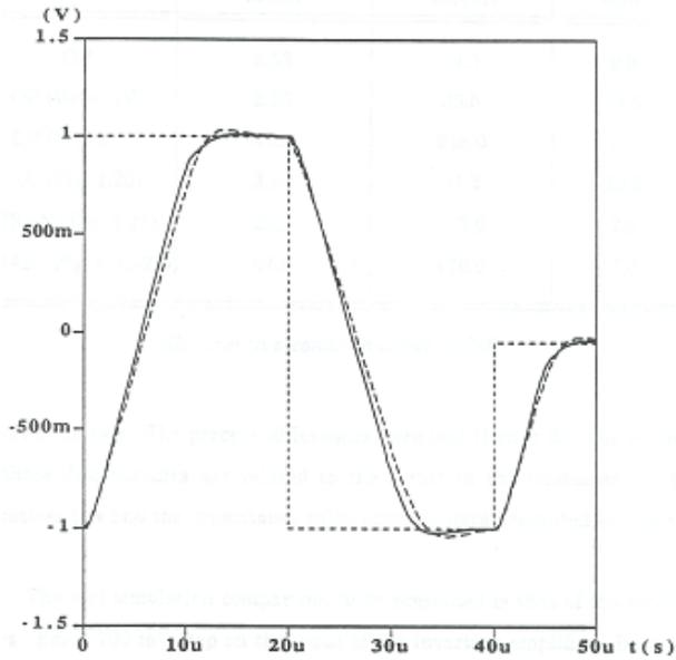
Figure 7. Large-signal transient response of the op-amp and its behavioral model in a voltage follower configuration.
