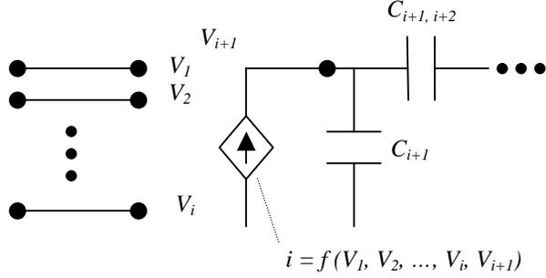
Figure 3. General representation of a physically modeled node.
