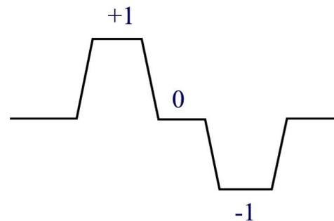
Figure 2: MLT-3 Encoded Waveform
