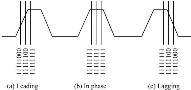
**Figure 10:** Phase Detection for Clock Recovery
