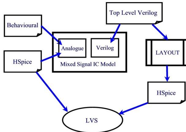
Figure 4: Modified IC Design Process Flow Diagram
