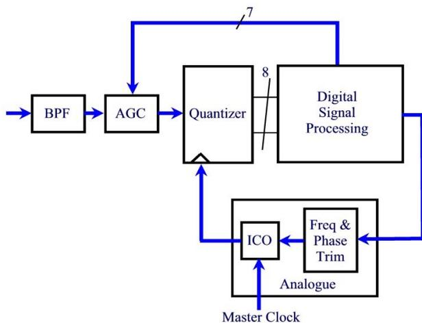
Figure 3: Receive Channel Clock Recovery
