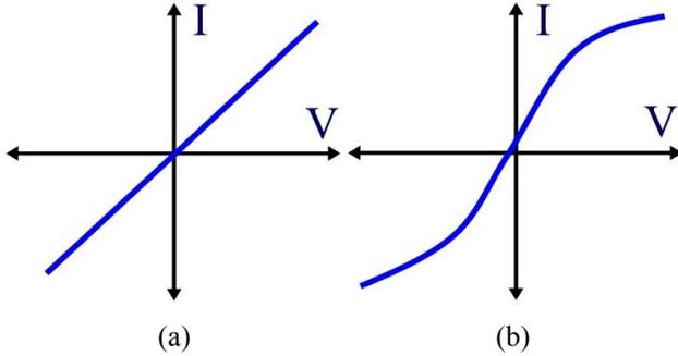
Figure 5: Gm Stage Characteristics (a) Ideal (b) Non-Linear
