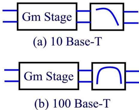
Figure 7: Gm Stage and Filter Model
