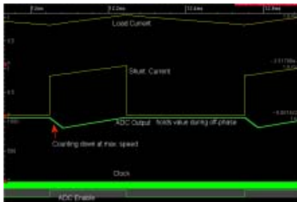
Figure 3 a: ADC holds output during off-state, Counting down at maximum speed after turn on
