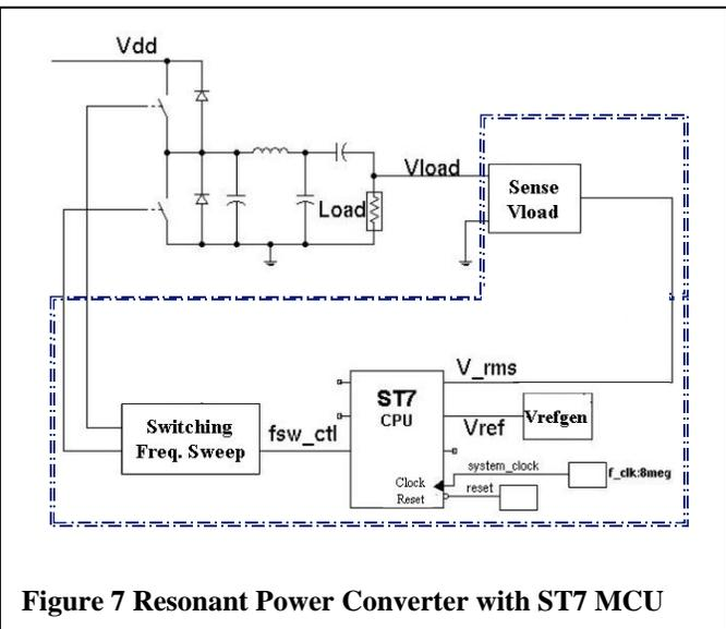
Figure 7 shows a resonant power converter schematic. The load voltage is regulated by modulating the switching frequency following a simple algorithm in the form.
