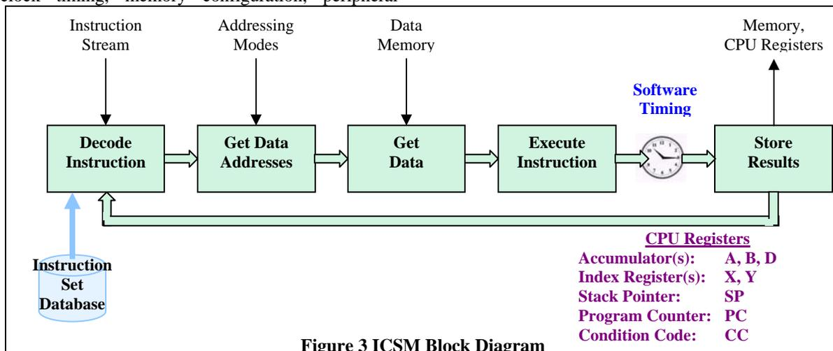
limited sequence of bytes in a local array and to refill that buffer as needed from memory. The instruction decoder keeps count of the number of bytes read for each instruction not only to refill the buffer but to set a pointer to the next instruction. This pointer is the preliminary update to the program counter. The instruction decoder algorithm accounts for the device-specific structure of the instruction stream which is generically in the form of:
