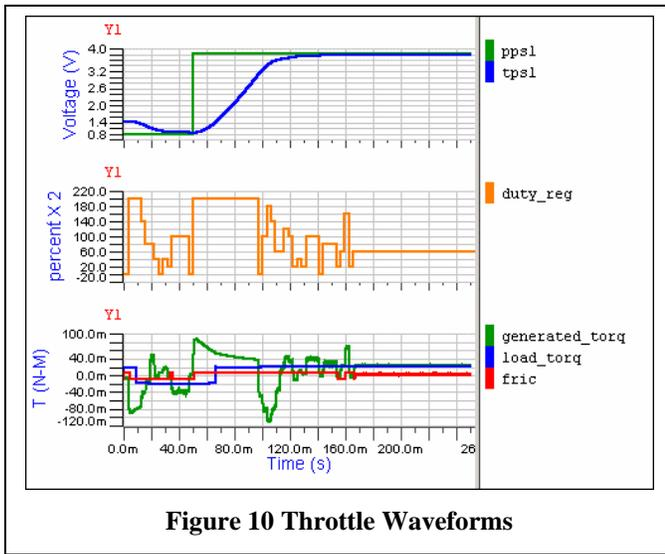
throttle for an embedded PID controller is plotted in Figure 10. Figure 11 shows an example in which the simulation is used to detect rounding errors due to the use of fixed point arithmetic. Embedded software relies on fixed-point computation to simultaneously reduce delays and program size.
