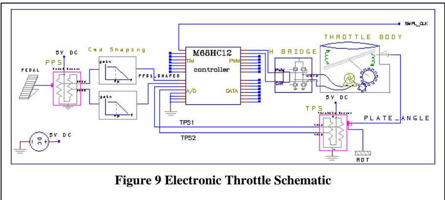
Figure 9 shows the schematic of an electronic throttle controlled by an HC12 MCU. The step response of the
