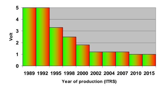
Need to reduce power supply voltage limited by:
