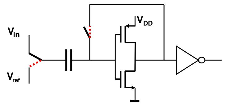
Removes off-set at the input, loses time
