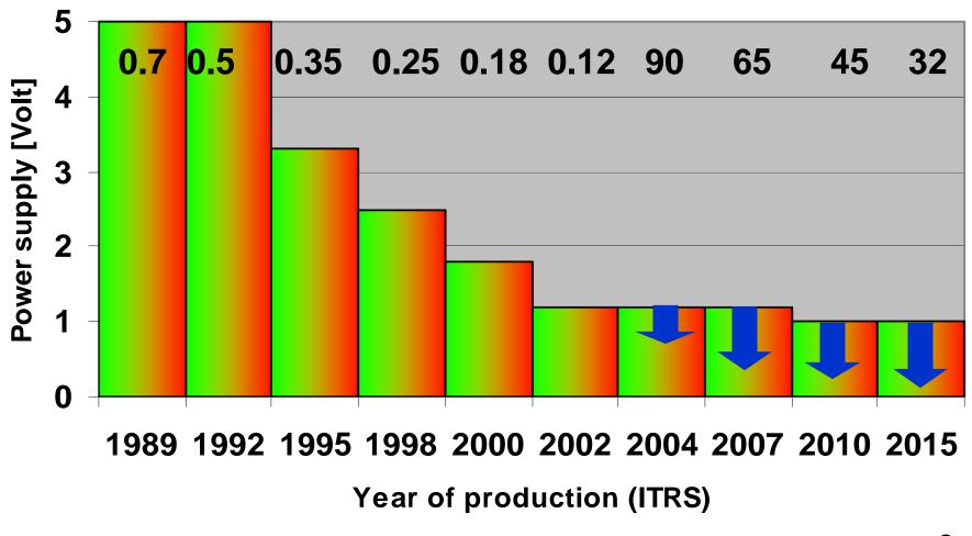
Power= activity x frequency x capacitance x **Voltage**<sup>2</sup>
