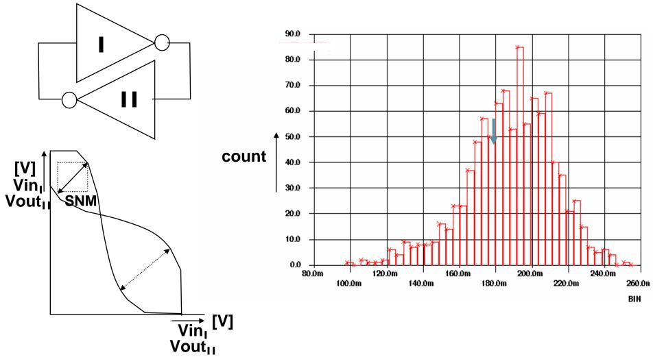
In SRAM 6T cells Static Noise Margin: size of "eye" defines robustness
