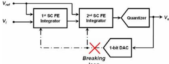
Figure 7. Extraction Mode of Second-Order SC  $\Delta\Sigma$  modulator
