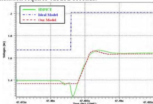
Figure 10. Output Timing Waveform of 1<sup>st</sup> Integrator
