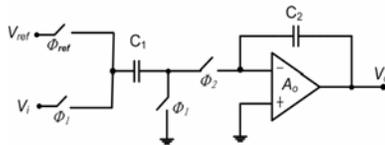
Figure 3. Single-ended Configuration of SC FE Integrator
