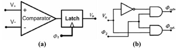
Figure 5. Schematic Circuit (a) Quantizer (b) 1-bit DAC
