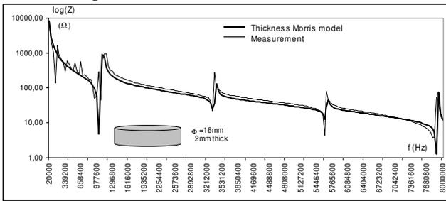
Fig 4: Impedance comparison between experiment and simulation for Thickness-mode Morris model
