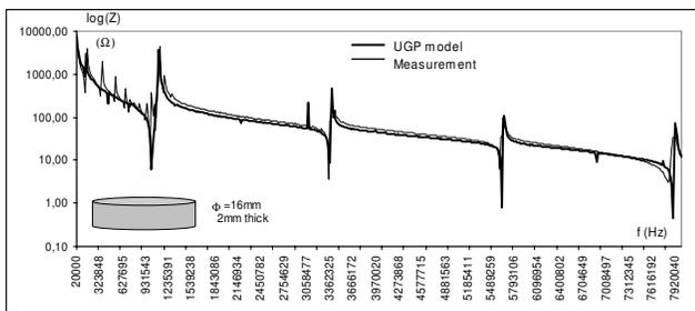
Fig. 10: Impedance comparison between experiment and simulation for the unified model (2mm thick)
