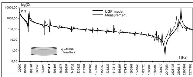
Fig. 11: Impedance comparison between experiment and simulation for the unified model (1mm thick)
