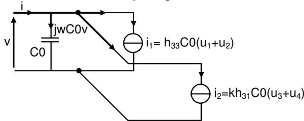
Fig. 7: Electrical part of the unified model
