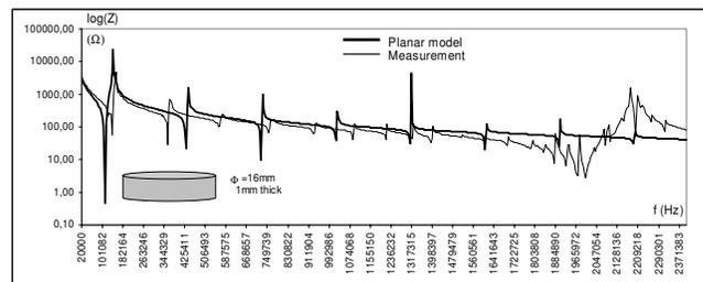
Fig 6: Impedance comparison between experiment and simulation for Planar-mode model
