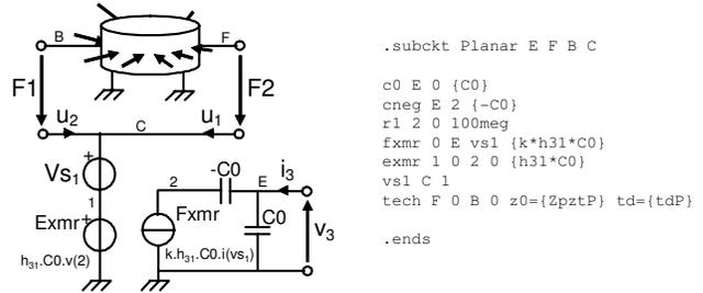
Fig. 5: SPICE planar mode transducer diagram and his corresponding SPICE netlist
