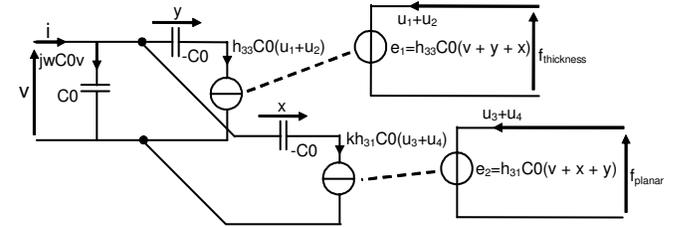
Fig. 8: Electro-mechanical part of the unified model
