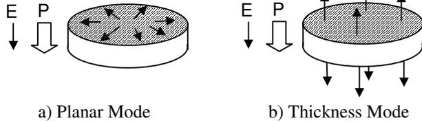
Fig. 1: Typical vibration modes of ceramic disks
