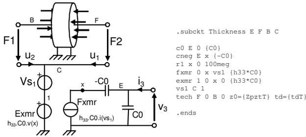
Fig. 3: Morris's SPICE thickness mode transducer diagram and his related SPICE netlist
