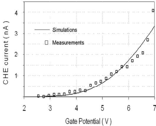
Figure 5:  $I_g$ - $V_g$  dummy cell characteristic with high  $V_d$ .
