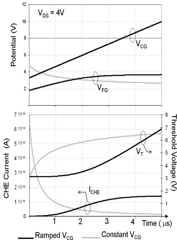
Figure 10: Simulations of the CHE programming operation by applying a ramped and a constant  $V_{CG}$ .
