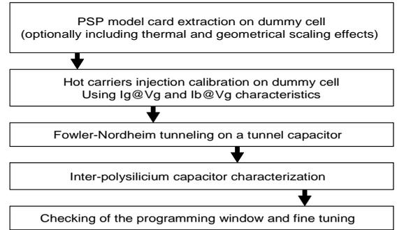
Figure 3: Characterization procedure diagram.
