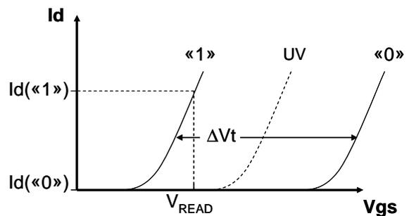
Figure 2: I-V curves of the Flash cell in erased, programmed and UV mode.
