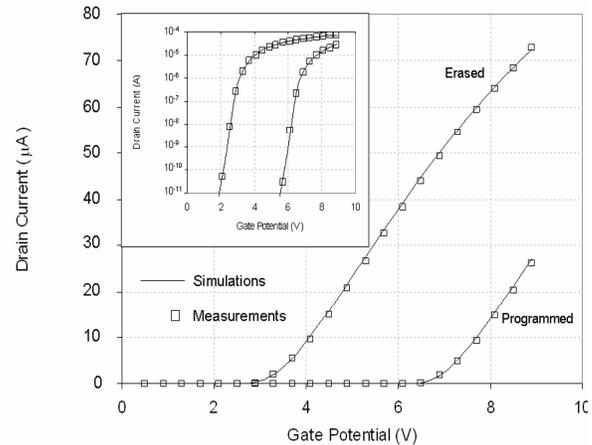
Figure 8: Drain current of the cell as function of control gate voltage in programmed and erased modes.
