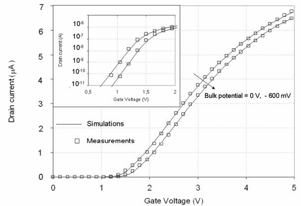
Figure 4: Id-Vg dummy cell characteristics.
