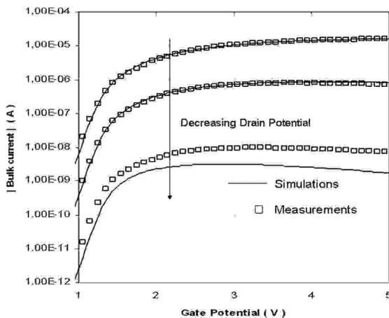
Figure 6:  $I_b$ - $V_g$  dummy cell characteristics.
