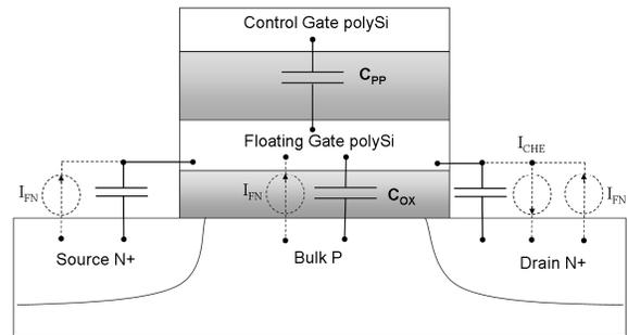
Figure 1: Capacitive structure and main injection currents of the Flash memory cell.
