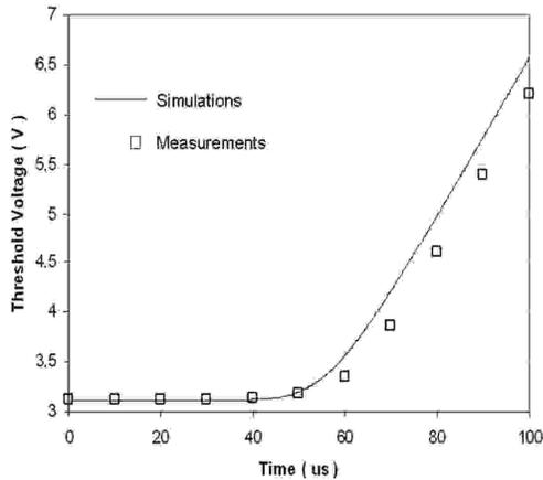
Figure 9:  $V_T$  evolution during a 100µs programming operation.
